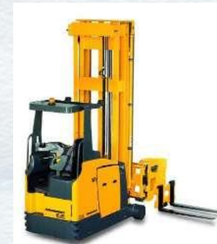
Narrow aisle truck
